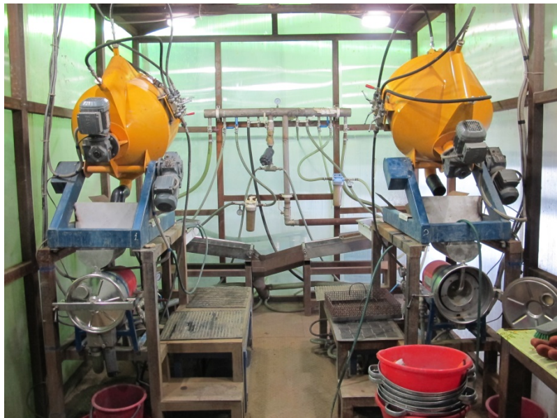
High-pressure trommel scrubbers integrated into a prospecting concentrator module (GROM)
