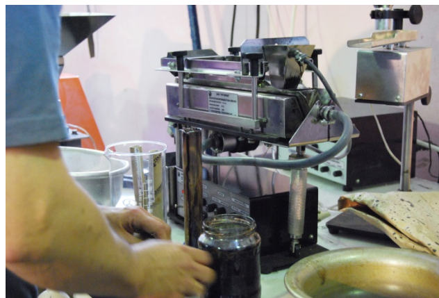
Magnetic liquid separator in action
