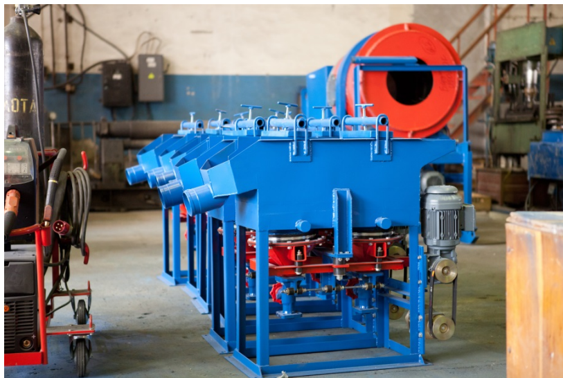
Jig MOD-02SK installed in a shop
